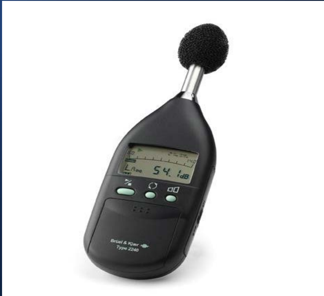
Low-cost integrating sound level meter
